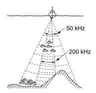
Figure 2-5 Comparisons of transducer frequencies
